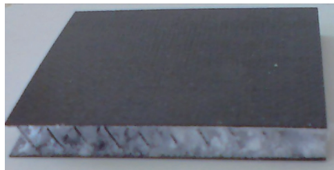
图1 X-cor夹层结构 Fig.1 X-cor sandwich structure
