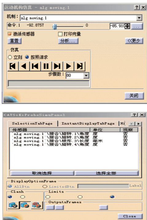
图9 DELMIA运动部件动态碰撞检测传感器 Fig.9 Interference check sensor for moving component in DPE
