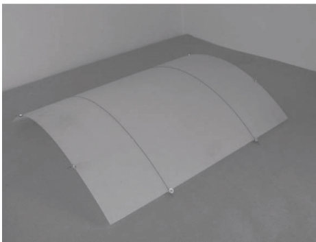
图1 预埋钛/镍(Ti/Ni)导线的双稳态结构 Fig.1 Titanium/nickel(Ti/Ni) wire circuit bi-stable knot
