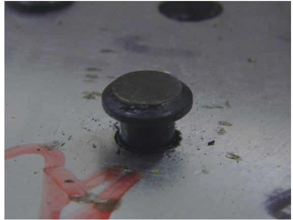
图2 采用风动铆枪在7050夹层结构中无法安装到位的高锁螺栓 Fig.2 Hi-lock bolt that can not be driven to stack by air gun
