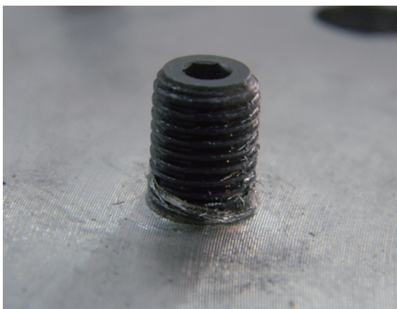
图1 采用风动铆枪在2024夹层结构中安装到位的高锁螺栓 Fig.1 Hi-lock bolt driven by air gun in 2024 aluminium alloy
