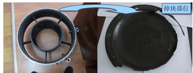
图3 排气段隔板与排气段完全脱落 Fig.3 Complete fall-off of drain clapboard and exhaust section
