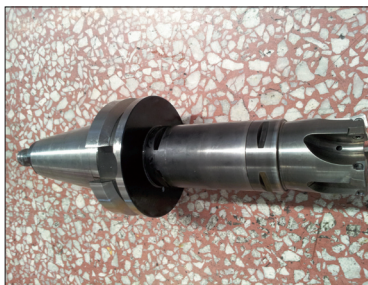
图8 试验用插铣用刀 Fig.8 Plunge-milling tool in test
