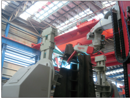
图5 机架的双机器人焊接 Fig.5 Dual robot welding of frame
