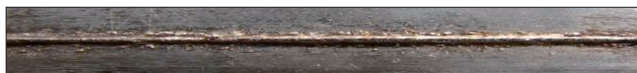
图 1 TC18 钛合金电子束焊缝背面成形( \delta=18\text{mm} ) Fig.1 Excess weld metal of electron beam welded TC18 ( \delta=18\text{mm} )
