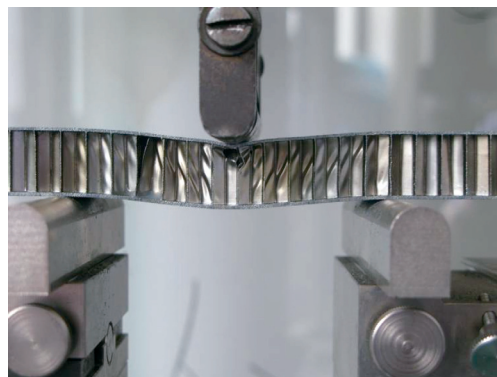
图4 3点弯曲试验 Fig.4 Three-point bending test
