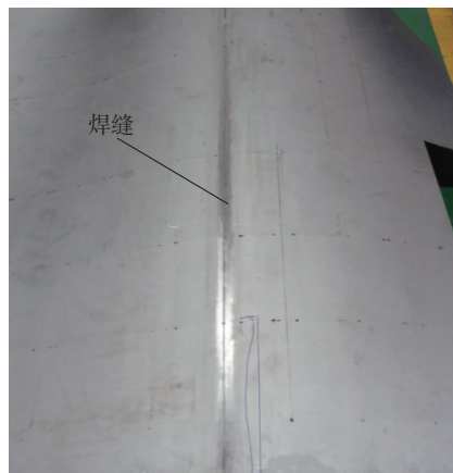
图9 单激光束熔焊整体蒙皮工艺样件 Fig.9 Sample of single laser fusion welding integrated panel
