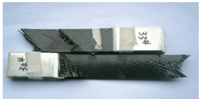
图3 疲劳试验件典型断口 Fig.3 Fatigue test pieces of a typical fracture
