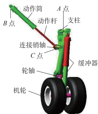
图1 飞机起落架虚拟样机模型 Fig.1 Virtual prototype of landing gear system
