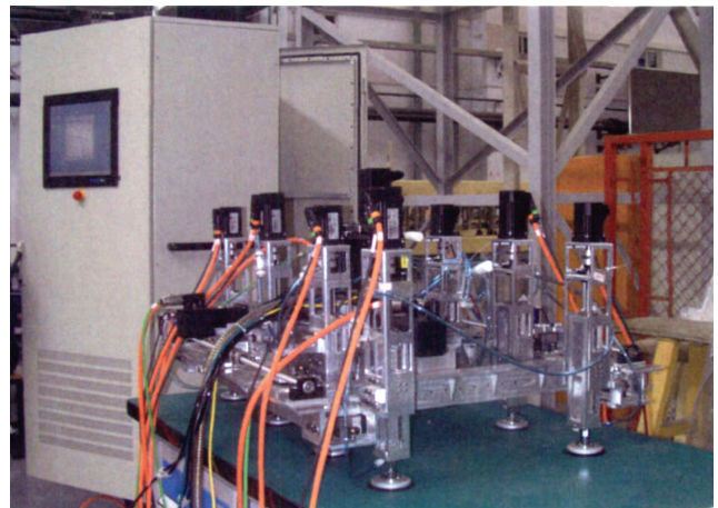
图5 南航等研发的爬行机器人制孔系统 Fig.5 Crawler robot drilling system developed by NUAAC etc.
