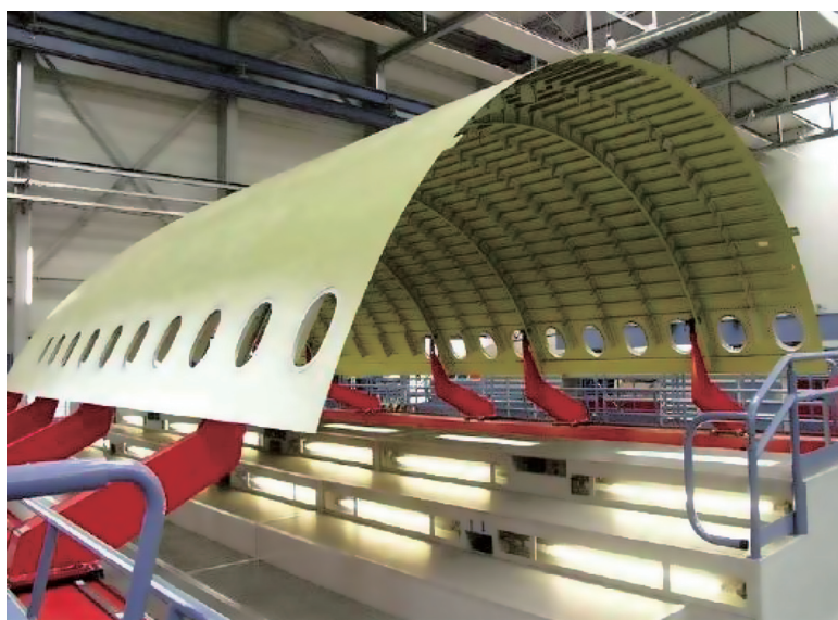
图1 A380上的Glare整体蒙皮 Fig.1 Integrally stiffened skin of Glare on A380
