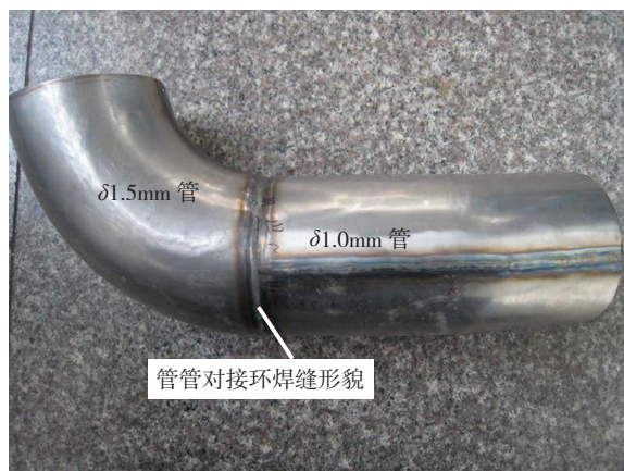
图6 环焊缝形貌 Fig.6 Macrostructure of circumferential weld
