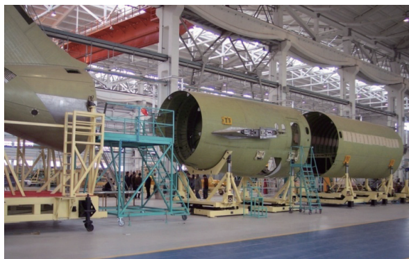
图2 ARJ21手动定位工装 Fig.2 ARJ21 manual locating tooling
