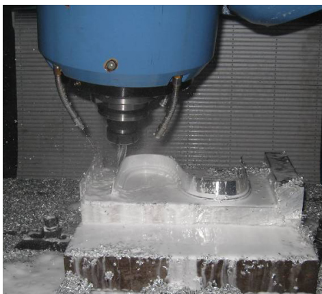
图3 “S”形试件加工测试 Fig.3 Detection of S-shape test-piece
