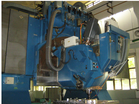
图1 AB双摆角数控铣头 Fig.1 AB bi-rotary NC milling head
