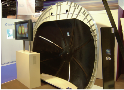
图1 空客A380复合材料后压力框 Fig.1 Composites rear pressure bulkhead of Airbus A380
