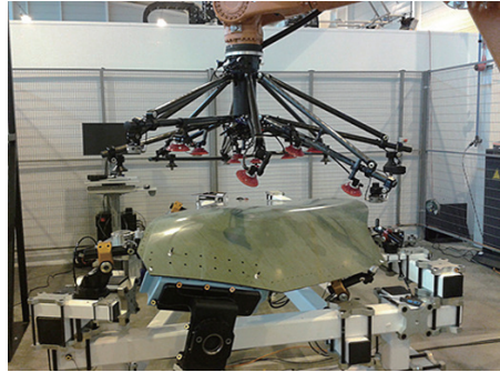
图3 GKN航宇公司机翼结构自动化装配 Fig.3 Automated assembly for wing structure in GKN Aerospace
