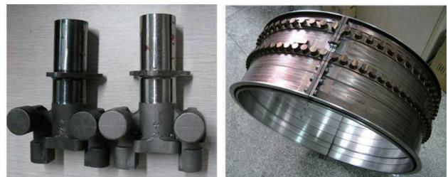
图3 西北工业大学采用LSF技术修复的航空发动机零件 Fig.3 Aeroengine components repaired using laser solid forming technology by Northwest Polytechnical University
