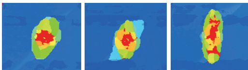
图2 各试件冲击后的C扫描损伤图形 Fig.2 C-scan damage of specimen after impact
