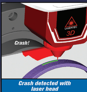
Collision detected between tool & additive part
