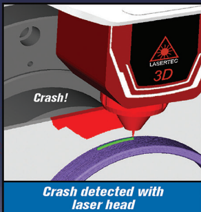
Collision detected between tool & additive part
