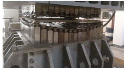
图7 三维数控弯板机冲压 Fig.7 Stamping by 3D CNC plate bending machine
