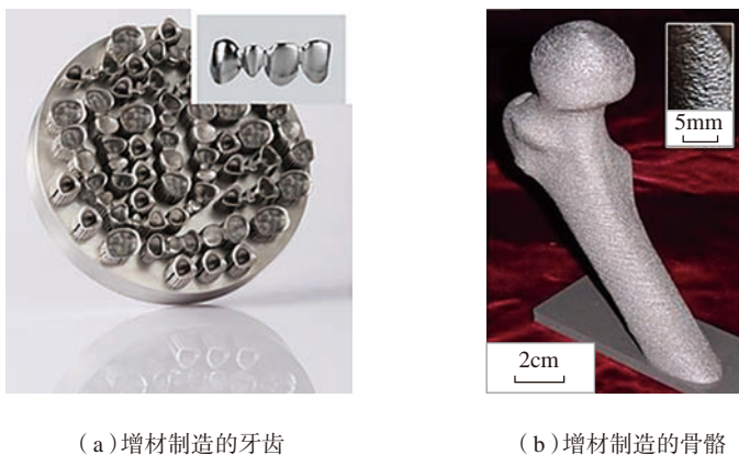
图4 增材制造在齿科、骨科方面应用 Fig.4 Additive manufacturing applications in dentistry and orthopedics
