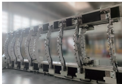
图11 飞机壁板柔性装配工装 Fig.11 Flexible assembly tooling for aircraft panel
