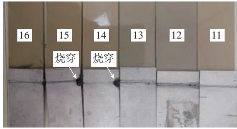
图2 2195 铝合金(表面未处理)- 聚醚醚酮激光连接试样 Fig.2 Laser direct joints of aluminum (surface untreated) and PEEK
