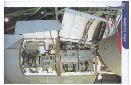
图1 典型的飞机舱位操作空间限制 Fig.1 Typical example of operations constraints in a limited aircraft bay
