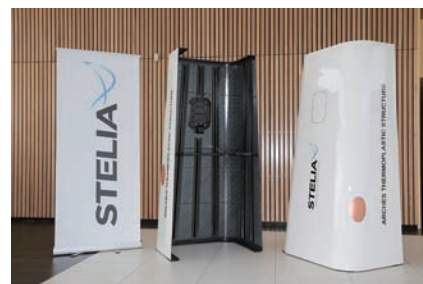
图9 Stelia公司研制的CF/PEEK热塑性复合材料机身验证件 Fig.9 CF/PEEK thermoplastic composite fuselage demonstrator manufactured by Stelia
