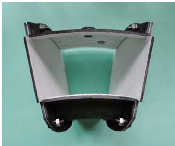
图1 BSAS涂层CVI-SiC f /SiC复合材料扇形燃烧室试验件 Fig.1 CVI-SiC f /SiC sector combustor liner with BSAS coating
