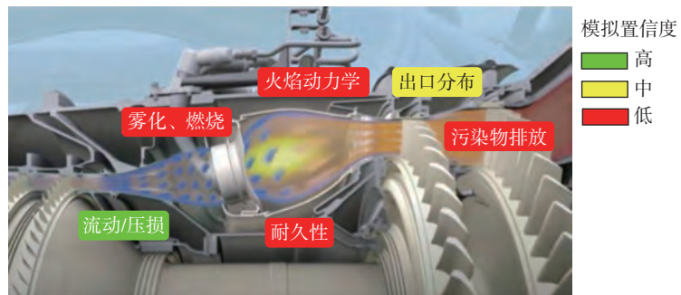
图2 燃烧室设计的关键问题以及现有模型、方法对于这些问题的预测置信度示意图 Fig.2 Schematic plot for some key issues of combustor design and the level of simulation accuracy for these issues
