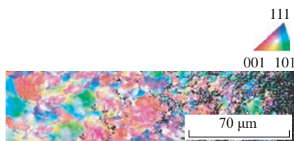
图30 316L不锈钢表面机械研磨处理后截面晶粒形貌 [65] Fig.30 Cross-sectional grains of 316L stainless steel processed by SMAT [65]
