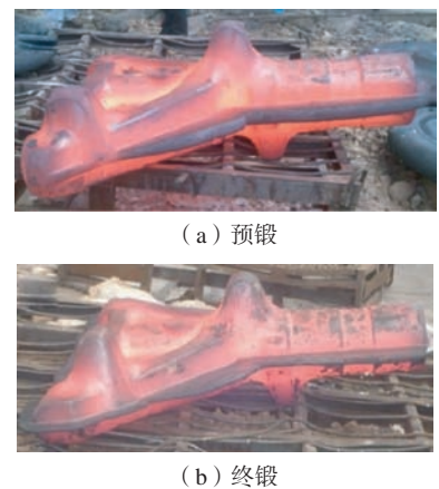
图3 飞机起落架外筒2火次模锻成形方案 [23] Fig.3 Two-stage die forging forming scheme of outer barrel of aircraft landing gear [23]
