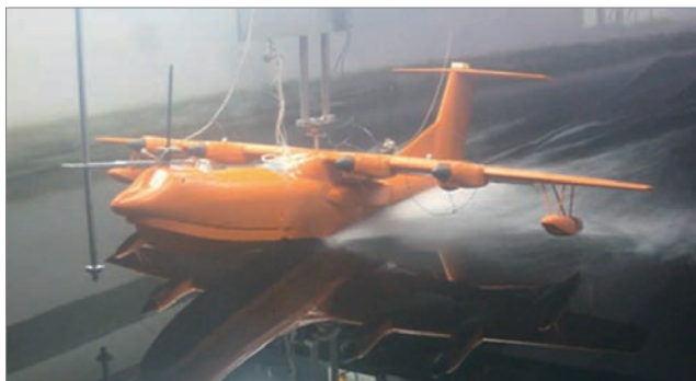
图 11 缩比模型着水试验 Fig.11 Pool test of scaled model
