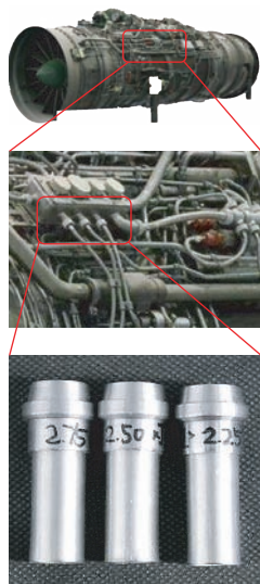
图 1 航空发动机油路密封管件 Fig.1 Aero-engine oil sealing pipe fitting
