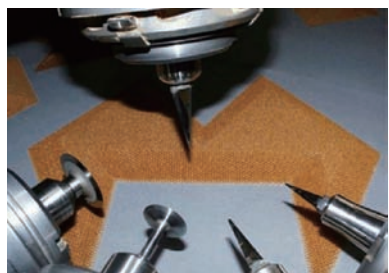
图 15 蜂窝芯超声加工刀具 Fig.15 Machining tools for ultrasonic cutting of aramid honeycomb core
