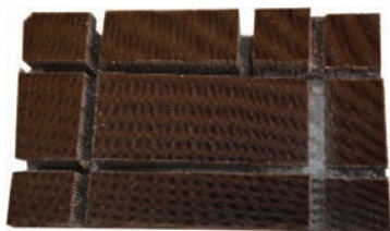
图8 一种蜂窝芯的凸台搭接固持方法 [51] Fig.8 A method for holding honeycomb core parts with false boss [51]
