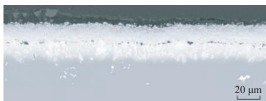
(a) 0.3 MPa/10 s-DZ125-5 \mu\text{m} -870 ^{\circ}\text{C} 渗铝
