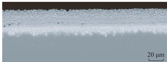
(c) 0.1 MPa/5 s-DZ125-5 \mu\text{m} -870 ^{\circ}\text{C} 渗铝
