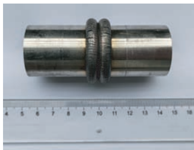
图3 GH4169 焊接接头宏观形貌 Fig.3 Macro morphology of IFWed joint of GH4169
