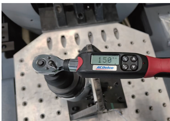
图 17 试验件螺纹预紧力矩设置 Fig.17 Thread pre-tightening torque set-up of test article
